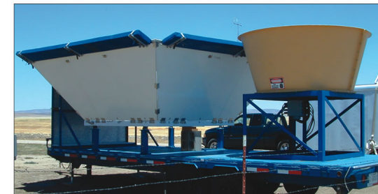
SODAR Sonic Detecting And Ranging 40 – 600 m 20 m Schichtung
